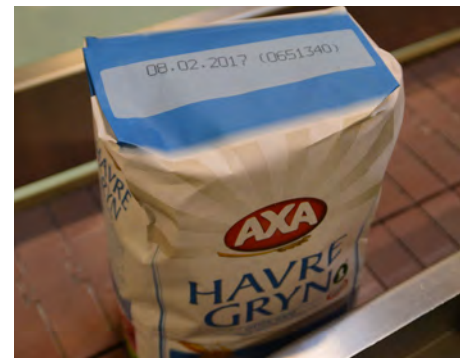
A new code was developed for implementation with CodeIT Enterprise and improves traceability to the minute in the packaging factory.
